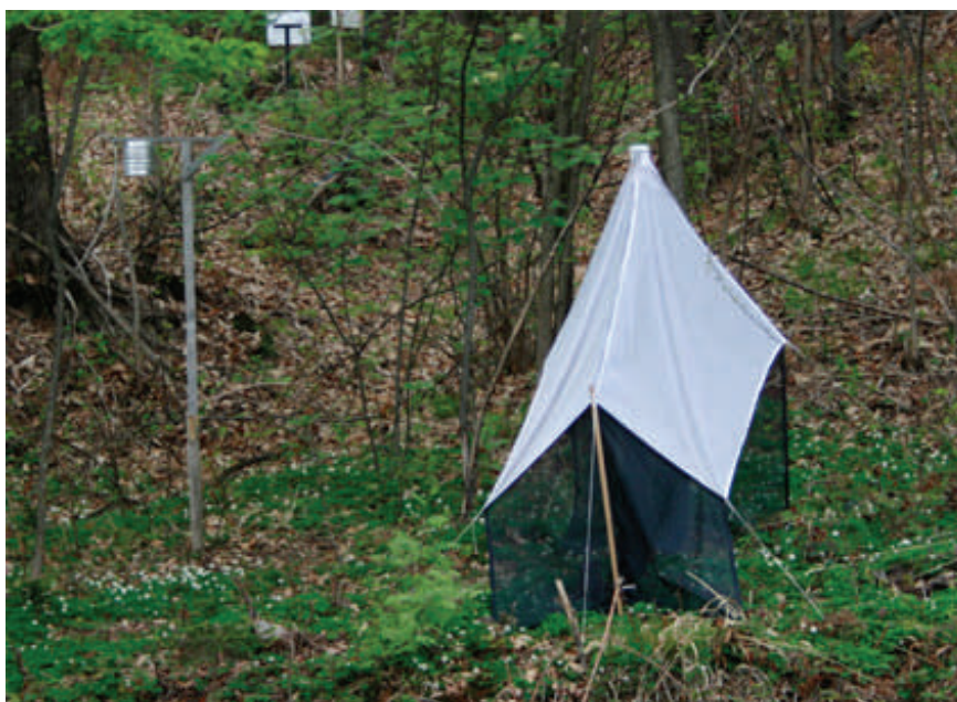
Photo 1: Malaise trap for catching hoverflies and other flying insects. Left from the trap is a temperature logger to measure temperature during the whole catching period. (Photo: A. Verlič)
