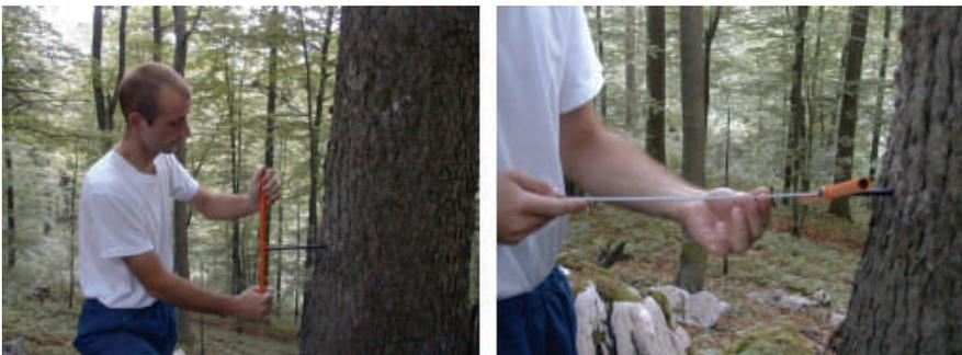
**Figure 3:** Sampling trees using incre- ment corer (or Pressler's corer).
