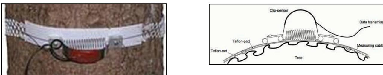
**Figure 1:** Schematic presentation of the circumferential electronic dendrometer D6 produced by UMS Munich, Germany (right) and the same dendrometer installed on a tree (left). White plastic beneath the dendrometer is super-smooth Teflon plastic, which allows undisturbed movement of the Invar wire going around the stem of tree. Source of images: UMS Munich Internet photo archive.
