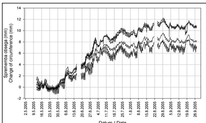
**Figure 2:** Typical sequence of electronic dendrometer measurements – increasing sinusoidal curve indicating radial growth and shrinking and swelling of the trunk in accordance with water availability. Beginning, period of most intensive growth and period of reduced growth is also visible.
